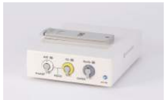
The AP-170P Hemodynamic unit supports PiCCO, ProAQT and CeVOX technologies with one unit.
